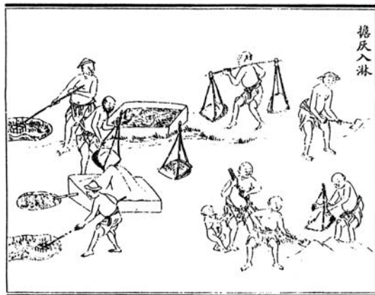
Salt in China. Fig. 1 Sea salt production from the Aobo tu of 1334, with the title “Carrying the ashes and pouring them into the leaching basin.”
